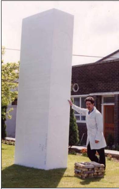
Before and After Compaction
