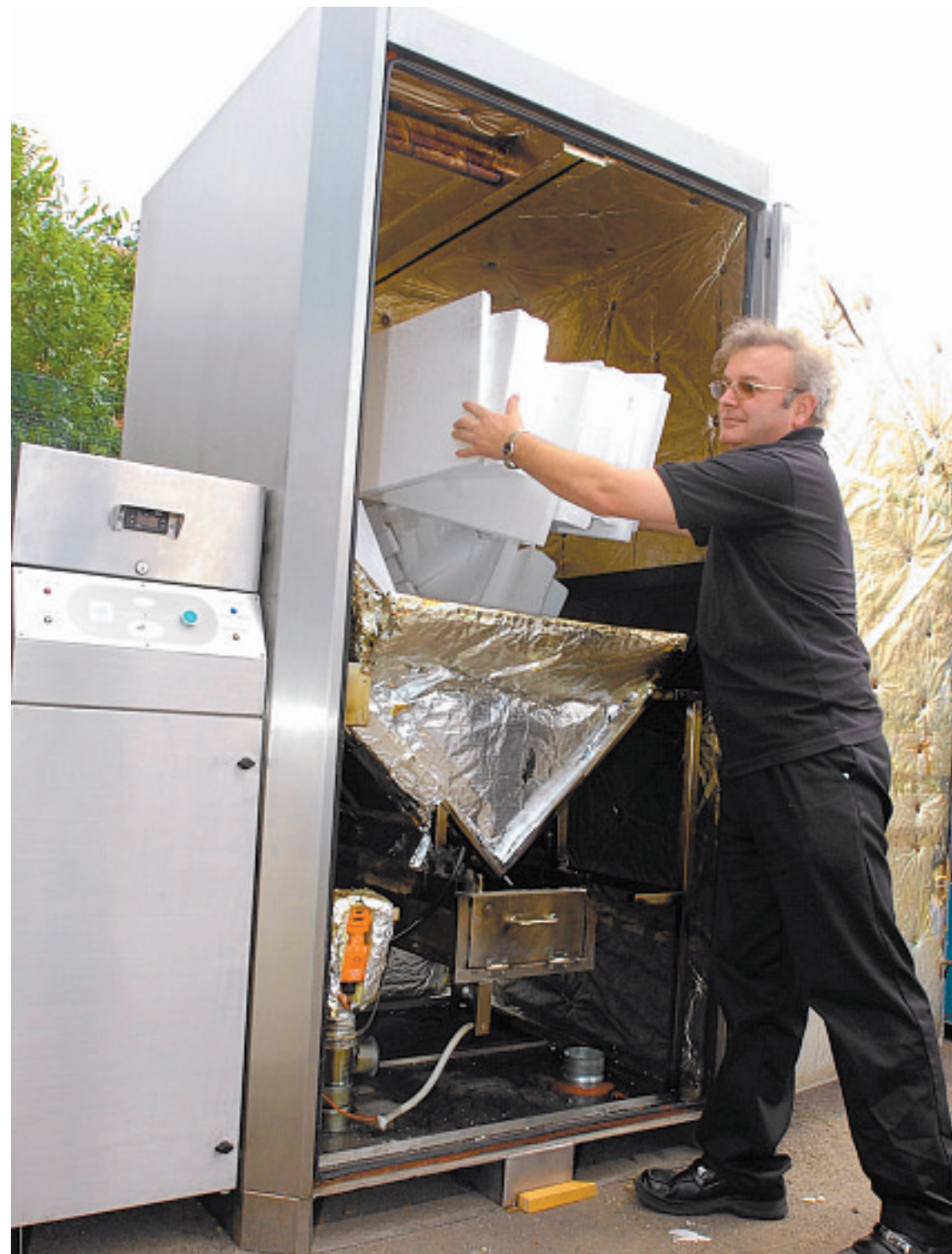
▲ Dealing with polystyrene mountain: Eric Butcher fills the Purex Styromelt machine ... and shows the much-reduced residue which can be put to a number of uses
